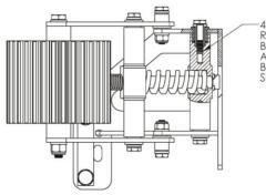
4X THREAD SEALANT REQUIRED ON THESE BOLTS BE CAREFUL NOT TO OVER APPLY AND GET SEALANT BETWEEN BUSHING AND SPACER
